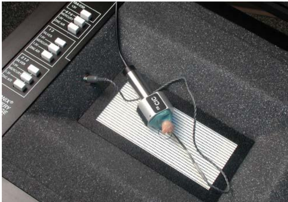
Figure 6 – Sealing a CIC hearing aid to a CIC coupler. Be sure to press [F1] “Coupler”; then [Menu], scroll down using the down ↓ arrow key to “Coupler type” and then the right → arrow key to “CIC” and press [Exit].
