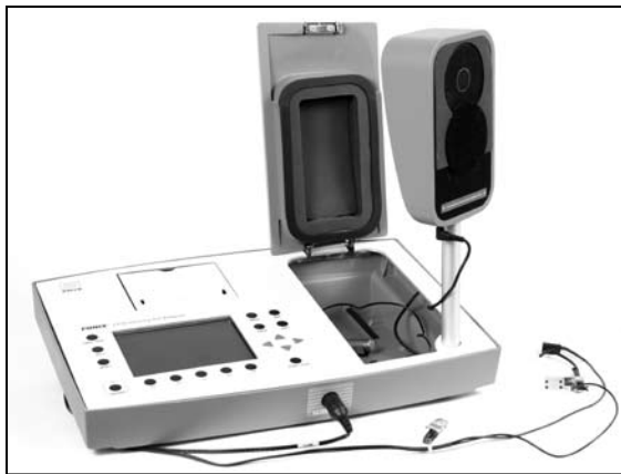
Figure 4.2.2—Internal sound field speaker setup
