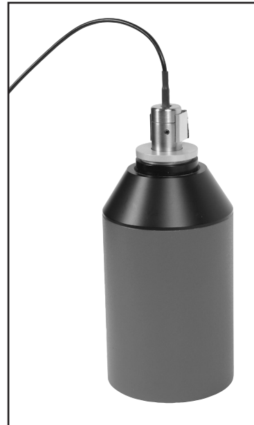
Figure 3.4.1: Coupler microphone inserted into sound calibrator.
