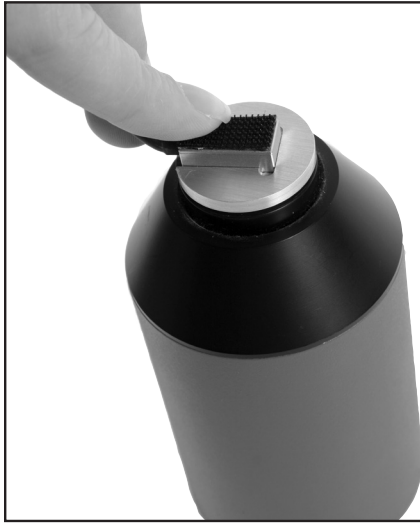
Figure 3.5.2A: Rectangular reference microphone inserted into sound calibrator.
