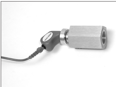
Figure 3.6.3A—Insert earphone connected to earphone calibration adapter and coupler
