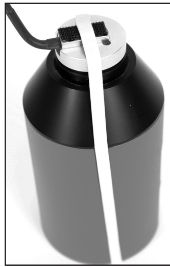
Figure 3.5.2B: Using a rubber band to hold the microphone in place on the calibrator.
