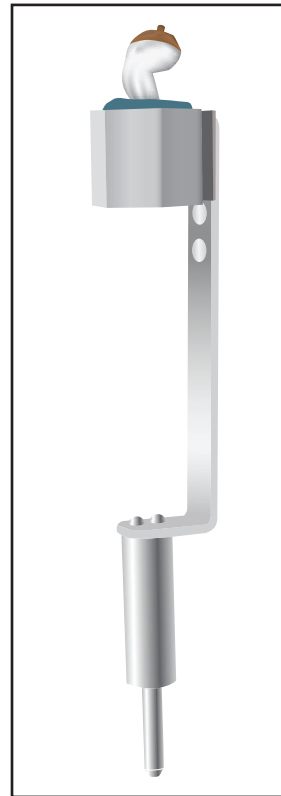
Figure 6.3.2B: Positioning the ITE hearing aid on the Rotating Shaft.
