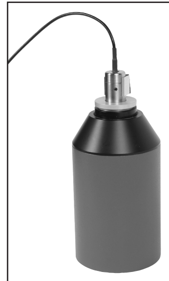
Figure C-2: Coupler microphone inserted into sound calibrator.
