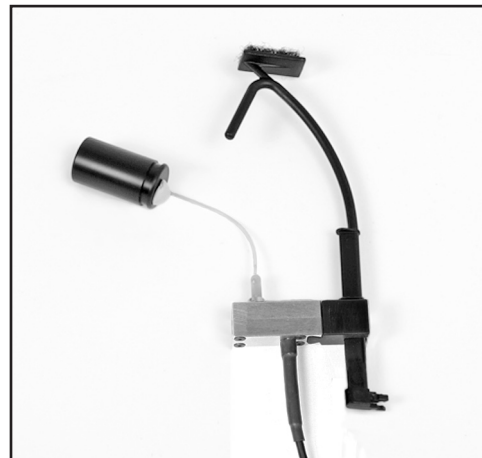
Figure 8.3.5B Probe tube in probe mic adapter
