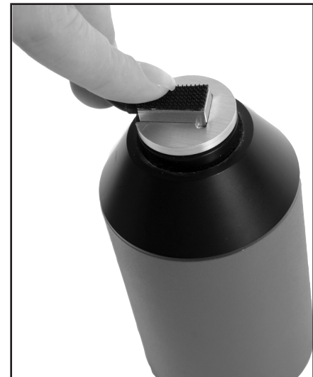
Figure C-4: Rectangular reference microphone inserted into sound calibrator.
