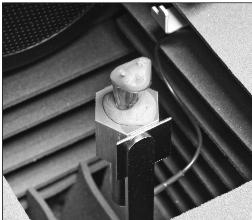
Figure 6.3.2C: Setting up an ITE hearing aid in the 8120 Polar Plot Chamber
