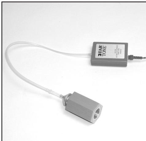
Figure 8.3.5A Insert earphone attached to coupler
