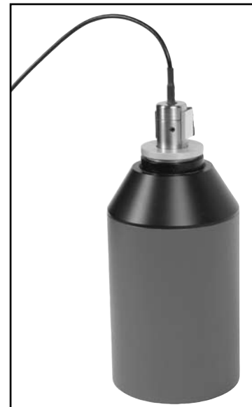
Figure B.1.1: Coupler microphone inserted into sound calibrator.
