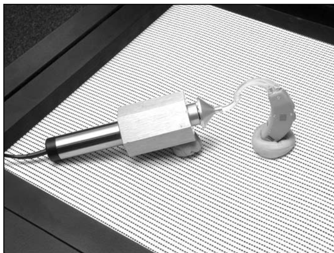
Figure 3.4.10A—Testing with the Sound Chamber Telecoil Board
