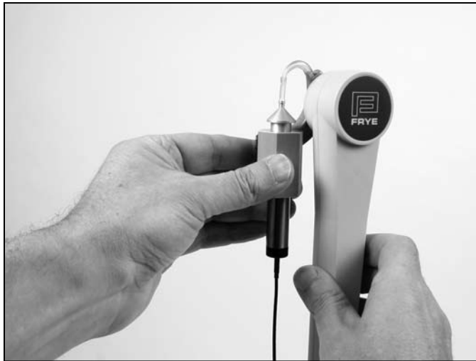
Figure 3.4.10B—Testing with the Telewand
