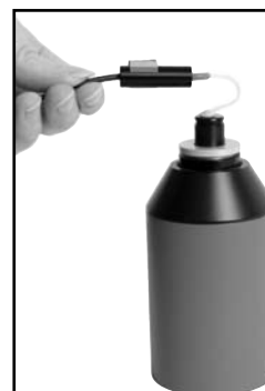
Figure B.1.2B: Old-style probe microphone inserted into sound calibrator.
