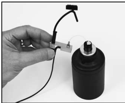
Figure B.1.2A: Integrated probe microphone inserted into sound calibrator.
