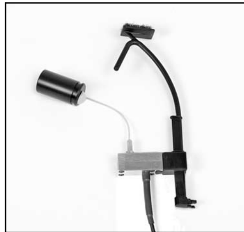
Figure 6.3.5B Probe tube in probe mic adapter
