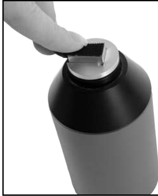
Figure B.1.3: Rectangular reference microphone inserted into sound calibrator.
