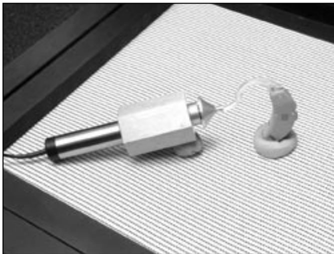
Figure 7.19.4—Telecoil measurement setup using the sound chamber's internal telecoil board
