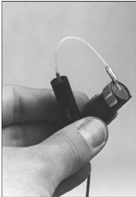
Figure 2.6.5A—Calibration clip holding probe tube in position
