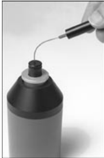
Figure 2.6.4B Probe microphone in calibrator
