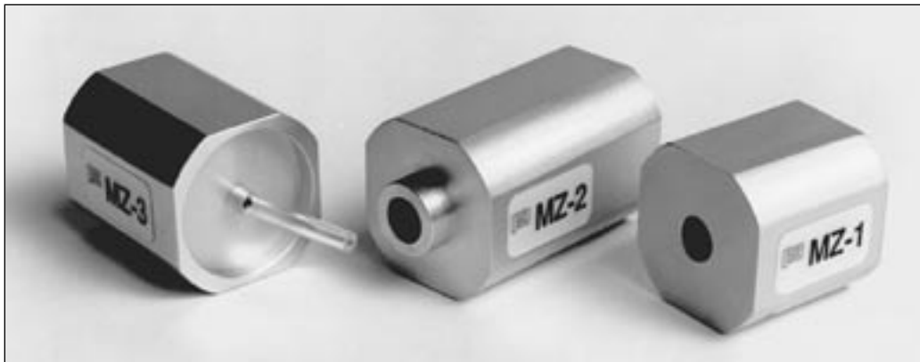
Figure 7.14.2A—Modified Zwislocki couplers used with OES and with IN-SITU
