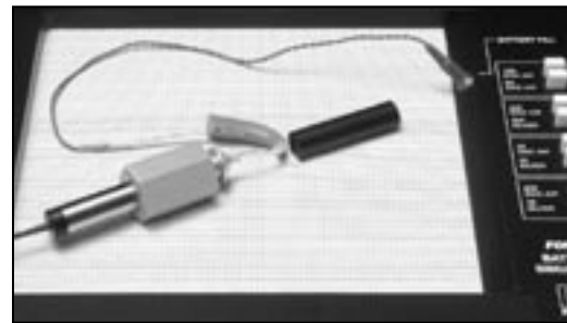
Figure 6.1.1B—Setup for aid testing/ equivalent substitution method
