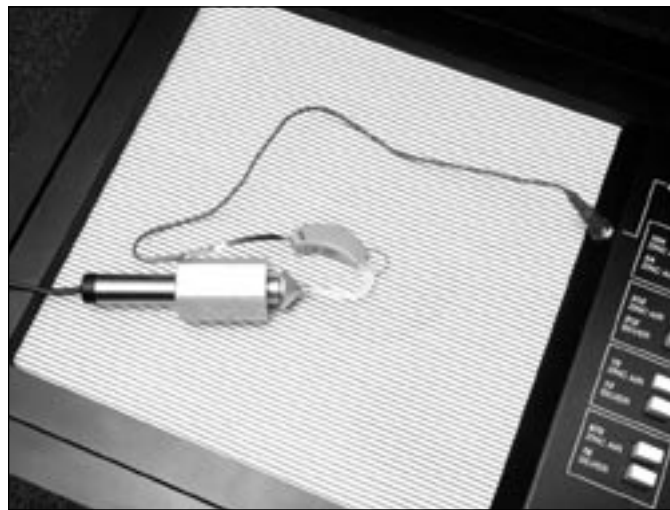
Figure 4.4 —Behind-the-ear aid with ear-level adapter
