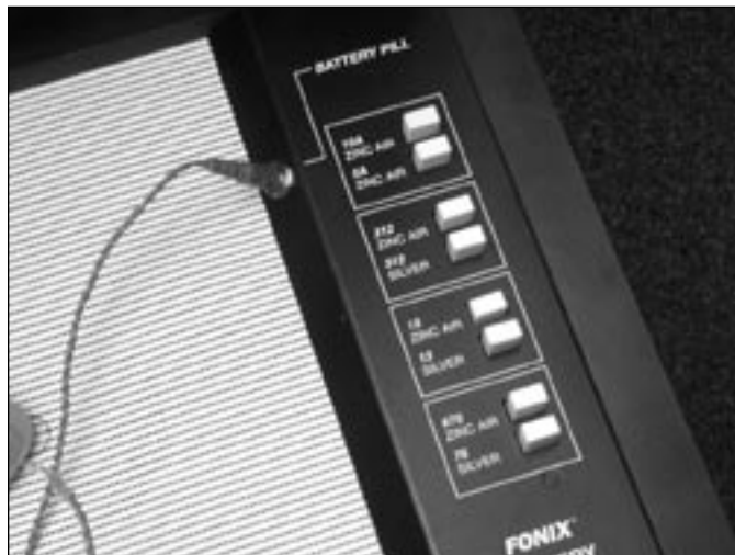
Figure 3.5.1—Battery voltage supply. Select the appropriate battery to simulate
